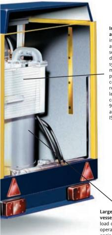
Improved compressed air quality by means of integrated aftercooler, automatic condensate separator and downstream reheating system. Additional microfilters make it possible to produce compressed air with a residual oil content of less than 0.01 ppm conforming to ZTV-SIB 90 standard, and other air quality standards to ISO 8573.1.
